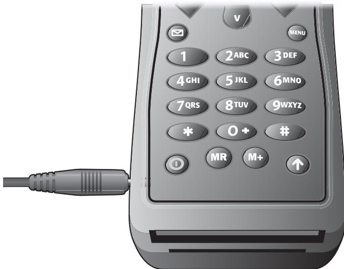
2. **Plug the travel charger** or auto accessory adapter into the appropriate power source. The phone beeps, flashes the
