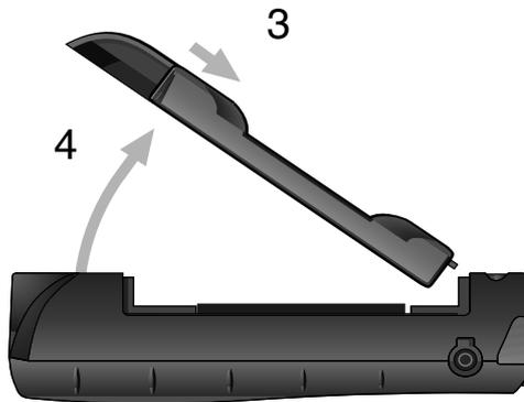
4. Pull the cover upward, and then remove it from the phone.
