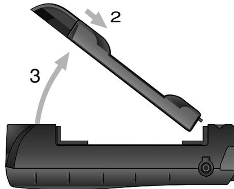
3. **Pull the cover upward**, and then remove it from the phone.
