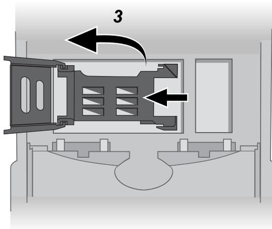
**4. Insert the SIM card into the tray with the notch up and the gold plate facing out.**
